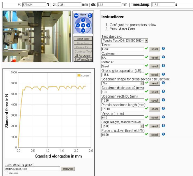
Figure 2. Tele-operated Tensile Test: real-time values (top bar); video stream with buttons to control and interact with the experiment (upper left); set-up panel for test configuration (right); real-time diagram including access to the test archive (left)
